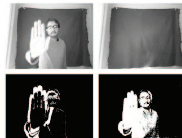
Prototype Four. Computer vision techniques for detecting motion and proximity
